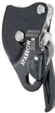
Self-braking descender for rope work, has been developed for high workloads. It allows the operator to lower themselves on the working line, to position themselves on it and to ascend the rope. It is ideal in the event of assisted lowering of two people with the device installed at the anchor (the operator lowers the rescuer and the person being rescued) or for simultaneous lowering of two people (rescuer lowers themselves with the injured person).
