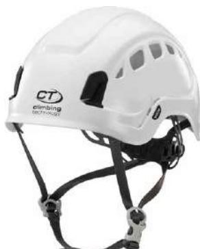
Ventilated helmet compliant with standard EN 12492:2012 and parts of EN 397:2012, which combined make it suitable for working at heights, rope access, tree climbing and rescue at heights services, including mountain rescue.
