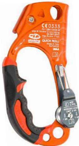
Innovative handled ascender, right or left-handed, with integrated pulley. Used in conjunction with a self-braking descender (e.g. Sparrow) it allows for easier ascents along the work rope.
