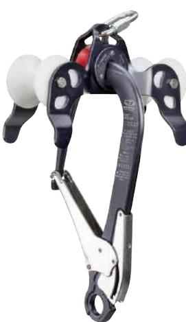
Combined anchor and pulley for evacuation from cable cars and chair lifts. It allows evacuation by allowing rescuers to be lowered along the cable, or when the underlying terrain permits it, to allow the unloaded pulley to run down the cable to the desired position and then use it as a winch and lower anchor.
