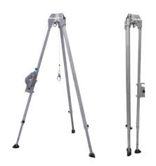
Portable tripod with adjustable locking legs and 3 intergated pullies. Head construction allows a variety of leg angles and a safetychain-free design. Ideal for economical compliance in many basic confined space, fall arrest applications and resuce.
