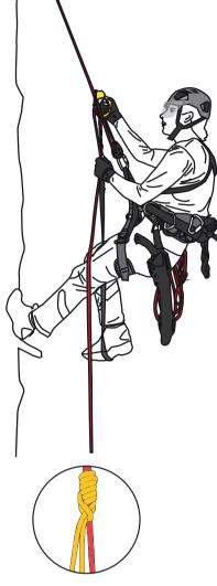
There are several methods of how to use rope techniques to get from the ground into a tree. One method is using a footlock.
