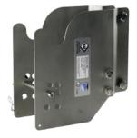
Stainless steel bracket designed to fit IKAR HRA recovery devices to IKAR Davit's mast. Bolts directly onto the davit' mast and comes complete with fixings and stainless -steel fixing pin for the device. Material: stainless steel 1.4571 (V4A) Dimensions: 264 x 162 x 250 mm (length x width x height) Weight: 3,5 kg (5 kg for HRA 33 version)
