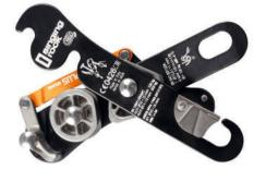
Manually operated descender device with double auto-locking system, that locks both when the lever is released or when it is pressed.
