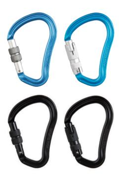
Large versatile pear-shaped HMS carabiner with screw/triple lock gate designed for multiple uses mainly for belaying or anchoring when working at height. Due to high strength and large gate opening it is mainly used as a central carabiner when anchoring.
