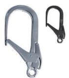
with double trigger automatic locking gate opening 110 mm • 25 kN polished, AI • 965 g • 34.04 oz unique production number C€ 0321 • EN 362
