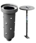
Flush floor sleeve with 3/8" drainage pipe connection to be installed to existing concrete by core-drilling and resin fix. A suitable shrink-free grout is PCI swelling mortar with the designation "Grout 100".
